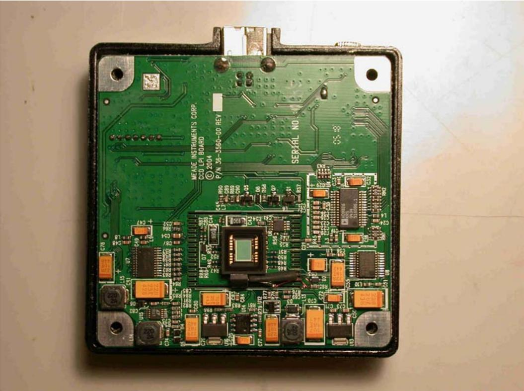
Fig.1 This is how the CCD-side of the DS1-Pro looks like. The sensor is mounted to the lower edge of the CCD
